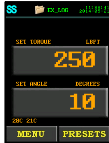
Figure 4.3.3-5: Main Screen with New Data Log Displayed
