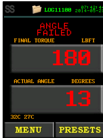
Figure 5.3-5: Failed Angle With the Bluetooth Bridge Disabled
