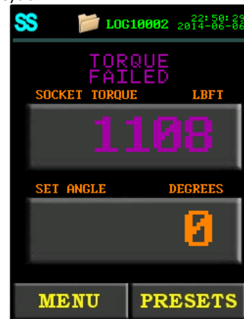
Figure 5.2-2: Failed Torque Cycle
