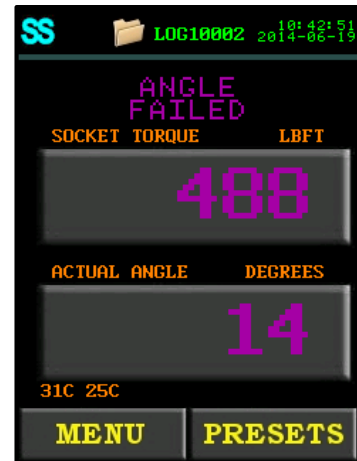
Figure 5.3-3: Failed Angle Cycle
