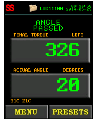
Figure 5.3-6: Passed Angle With a Smart Socket Not Connected
