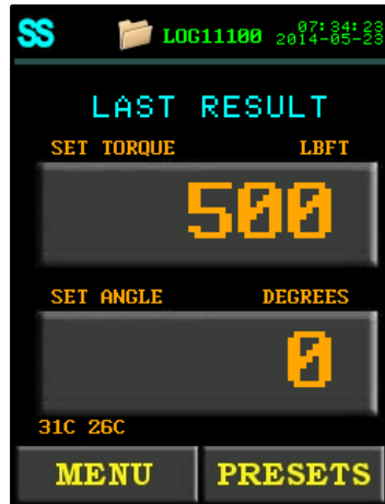
Figure 5.5-1: Passed Last Result With a Smart Socket Connected
