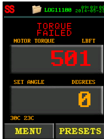
Figure 5.2-6: Failed Torque Cycle With a Smart Socket Not Connected
