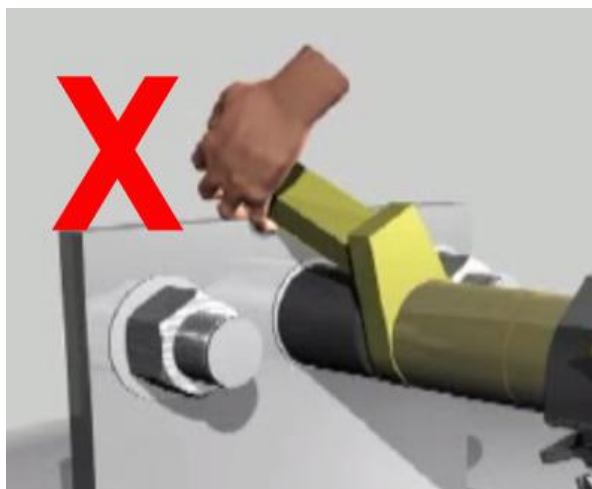
Figure 5.1.1-2: Incorrect Placement of Hand/Body Parts During Operation
