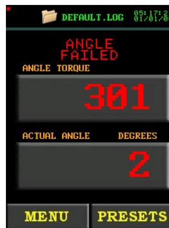
Figure 5.4.1-2: Failed Torque and Angle Cycle
