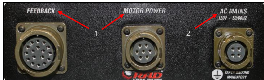
Figure 3.2-1: Controller Cable Connections
