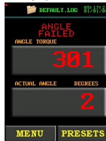
Figure 5.3-3: Failed Angle Cycle
