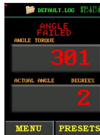
Figure 5.4.2-3: Failed Torque and Angle Cycle
