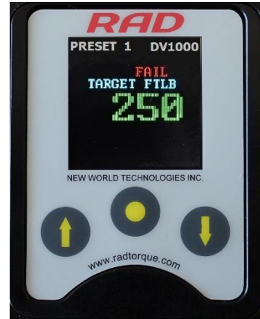
Figure 5.2-2: Failed Torque Cycle
