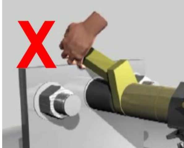
Figure 5.1.1-2: Incorrect Placement of Hand/Body Parts During Operation
