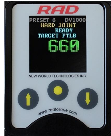
Figure 4.3.2-2: Main Screen – Hard Joint Mode
