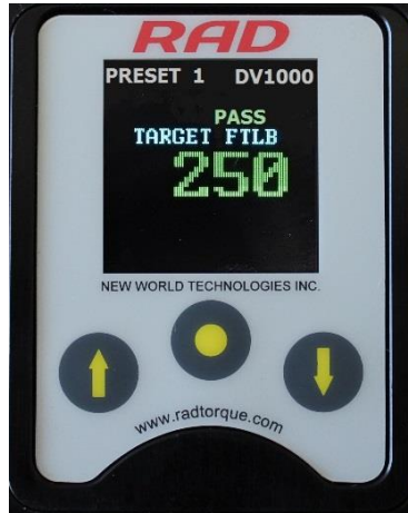
Figure 5.2-1: Passed Torque Cycle
