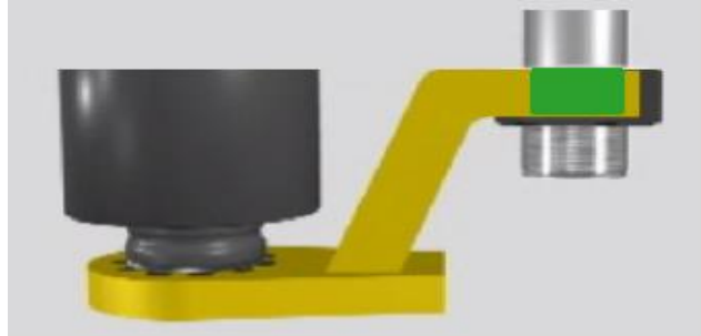
Figure 5.1.4-1: Correct Reaction Point
