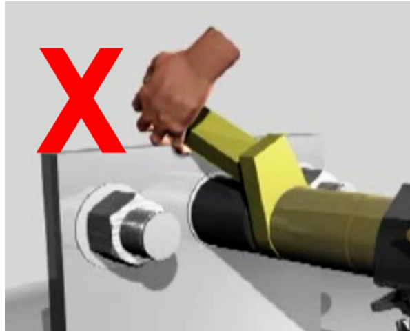
Figure 4.1.1-2: Incorrect Placement of Hand/Body Parts During Operation
