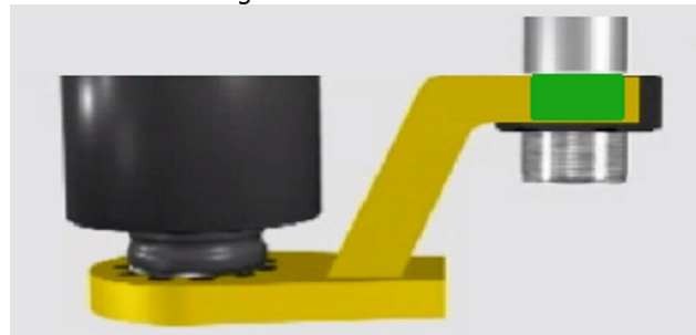
Figure 4.1.4-1: Correct Reaction Point
