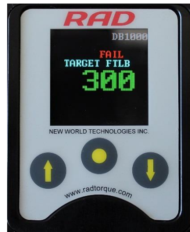
Figure 4.2-2: Failed Torque Cycle
